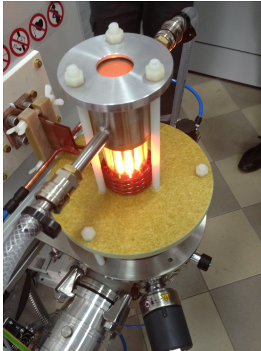
Fig. 3.3. Cold-chamber furnace, with vacuum and argon atmosphere
