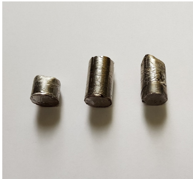
Fig. 5.1. Stainless steel ingots made in the induction furnace with a cold crucible
