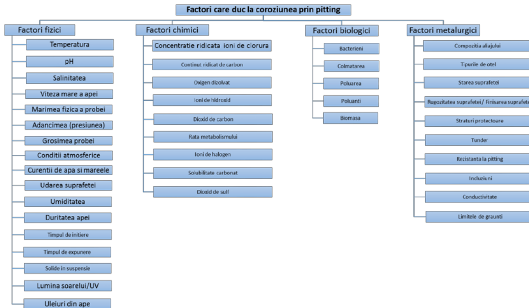
Fig. 2.1. Factors that can affect point corrosion
