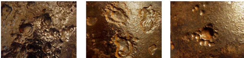
Fig.2 Terraced pitting specific of MIC
