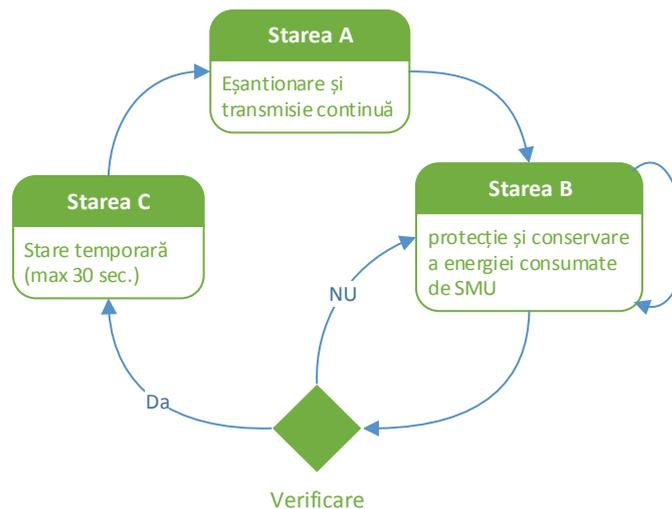
**Figura 22. The state chart of the storage management module within the SMU prototype (source: the author)**
