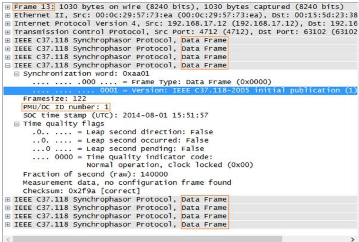
Figura 35. Validation of the fact that the PMU equipment within the WAMPAC network transmit the data unencrypted (source: the author, using the analysis tool Wireshark)
