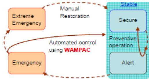
Figure 3. The state chart of a WAMPAC system (source: [16])
