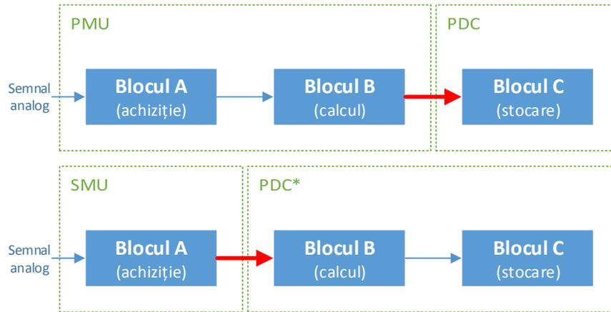
**Figura 20. The shift of the place where the data transfer takes place / difference between the PMU (up) and SMU (down) (source: the author)**
