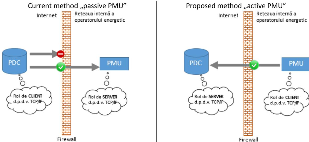
Figura 1. Comparison between the two implementation options for the communication topology between a PMU and a PDC within a WAMPAC system (source: the author)
