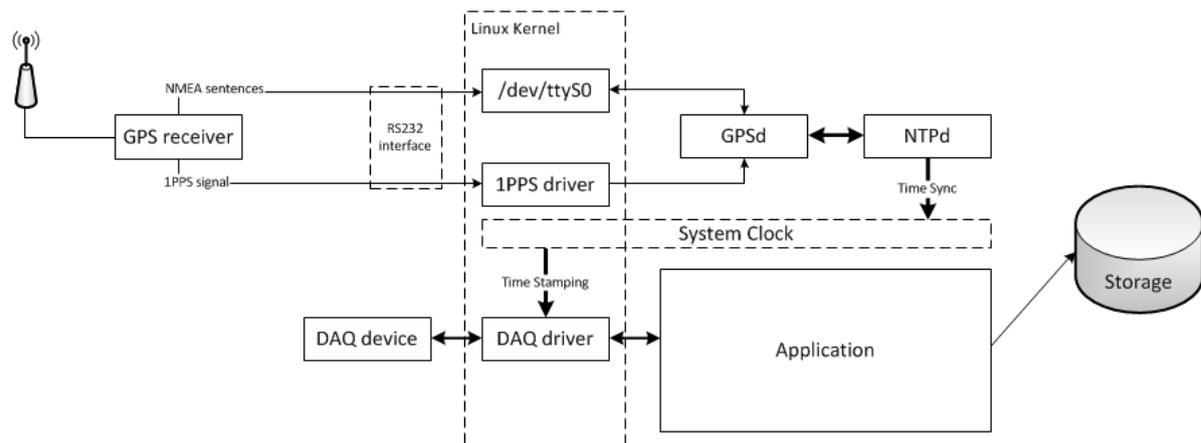
**Figure 7. Typical architecture of a GPS integration into a Linux operating system for synchronizing the internal clock (source: the author)**
