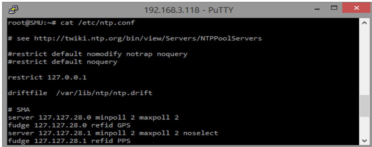
The image shows a PuTTY terminal window titled "192.168.3.118 - PuTTY". The terminal displays the output of the command "cat /etc/ntp.conf". The configuration file content is as follows:
