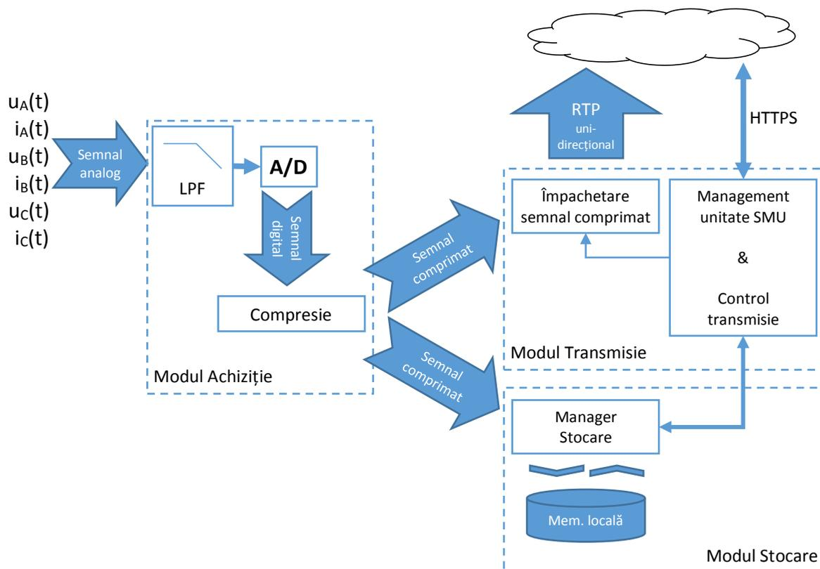
Figura 4. Processes run by the SMU equipment
