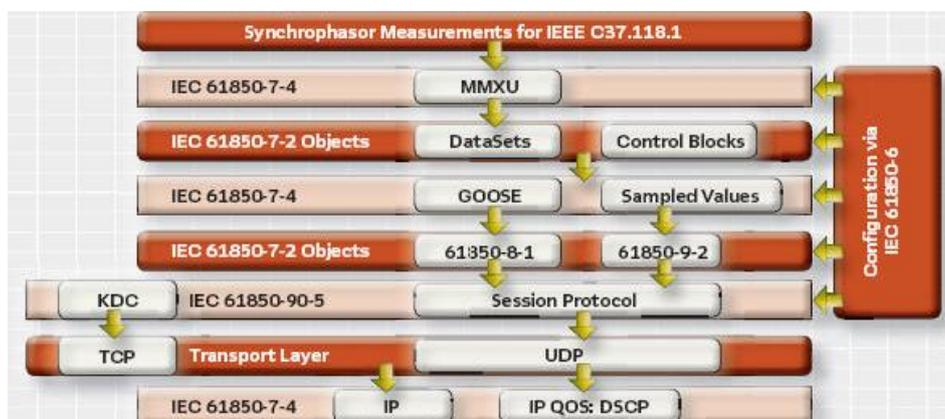
Figura 23. Integration between the C37.118 and IEC61850-90-5 (source: [31])
