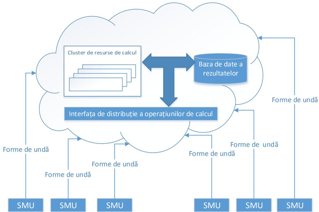
Figura 5. Concept of *cloud computing* used in the centralized computation of the power grip parameters based on the high definition waveforms delivered by SMU's (source: author)
