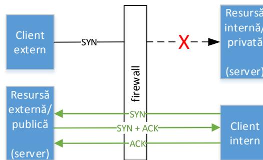
Figura 2. Difference between the connection initiated by from outside (blocked) and the inside one (permitted) (source: the author)
