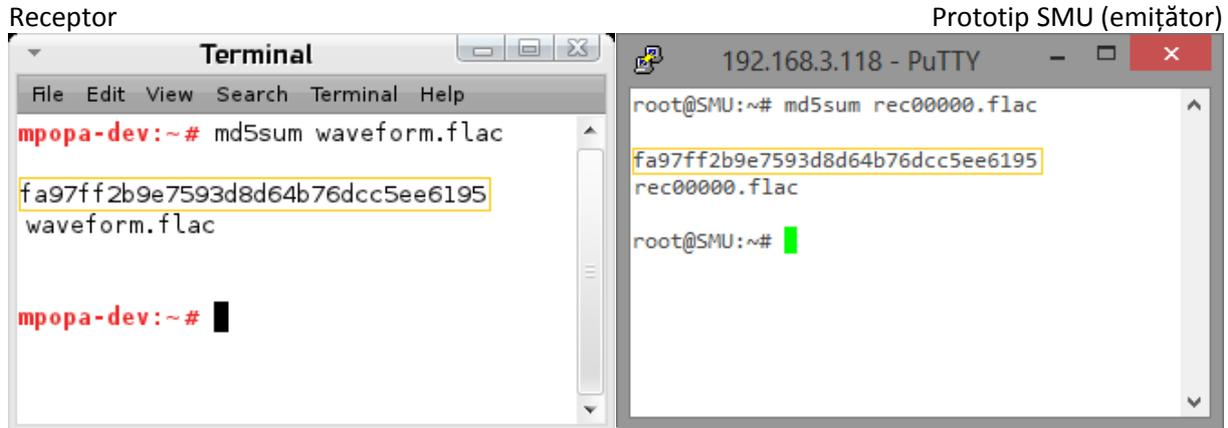
Figura 34. Validation of the fact that the transmitted waveforms by the SMU (right) and those received by the virtual machine (left) are identical (source: the author)
