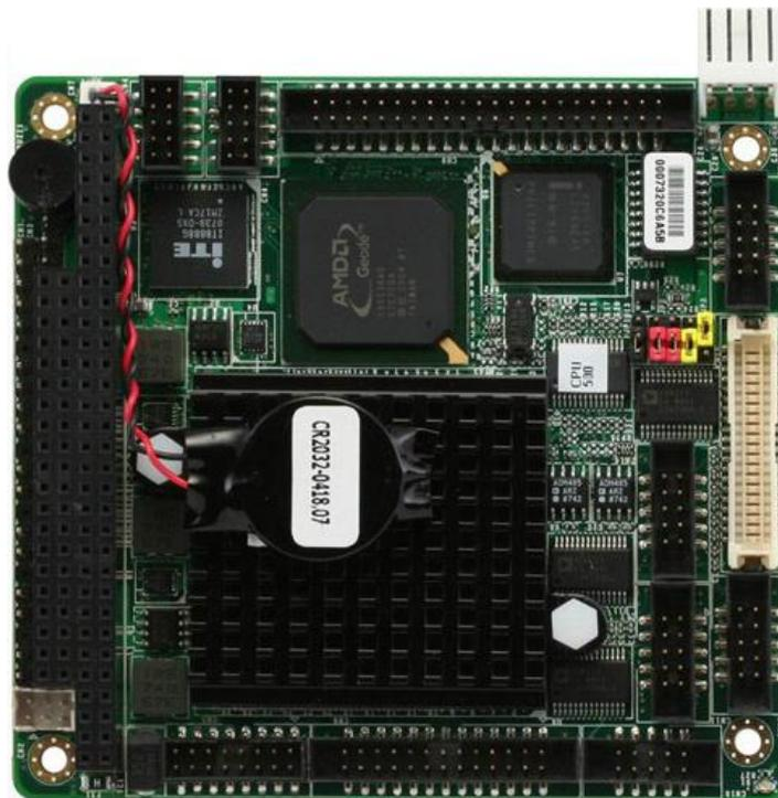
Figura 16. The SBC (single board computer) module used for the SMU prototype
