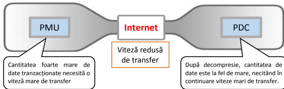
**Figura 15. The bottleneck problem, in case of systems with very high data flows.**
